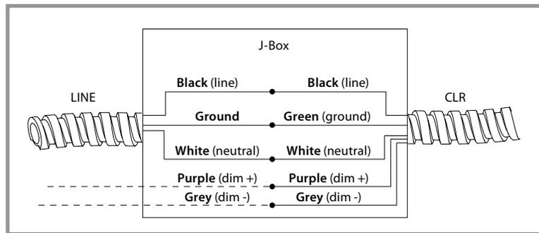
**NOTE:** If 0-10V dimming is NOT to be connected, it is recommended to cut off the exposed, tinned leads on the purple and grey wires, and cover the ends with a small piece of electrical tape or wire nut. If bare 0-10V control wires should accidentally touch a grounded surface, it could cause unintended flickering or dimming of the light fixture.
